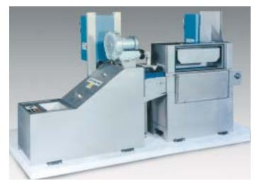
At unload, parts are stripped of excess solution by ambient air
